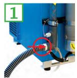
CONNECT THE OUTLET TUBE OF NITROX MIX FROM THE LP COMPRESSOR TO THE HP COMPRESSOR
