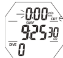
Fig. 70 - FREE SURFACE CDT ALARM
