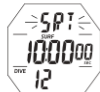
Fig. 71 - FREE SURFACE SRT ALARM
